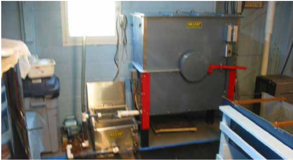
PHOTO 2. From left to right, the drip tank to hold uncapped honey comb, the extractor in the center, which empties into a baffle tank. To the right of the baffle tank is the honey pump.
